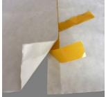
RadonProtect PREMIUM foil, the underside is laminated with fleece, with self-adhesive strips
